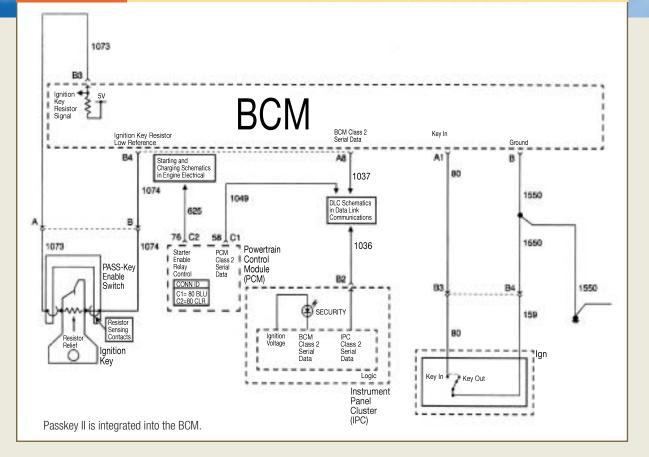
the first key inserted into the lock, it will recognize a key pellet in the same resistance range. Whether the TDM is a separate unit or built into the BCM, that key resistance range memory cannot be reprogrammed. The resistance range of that first key is what it will look for every time.
